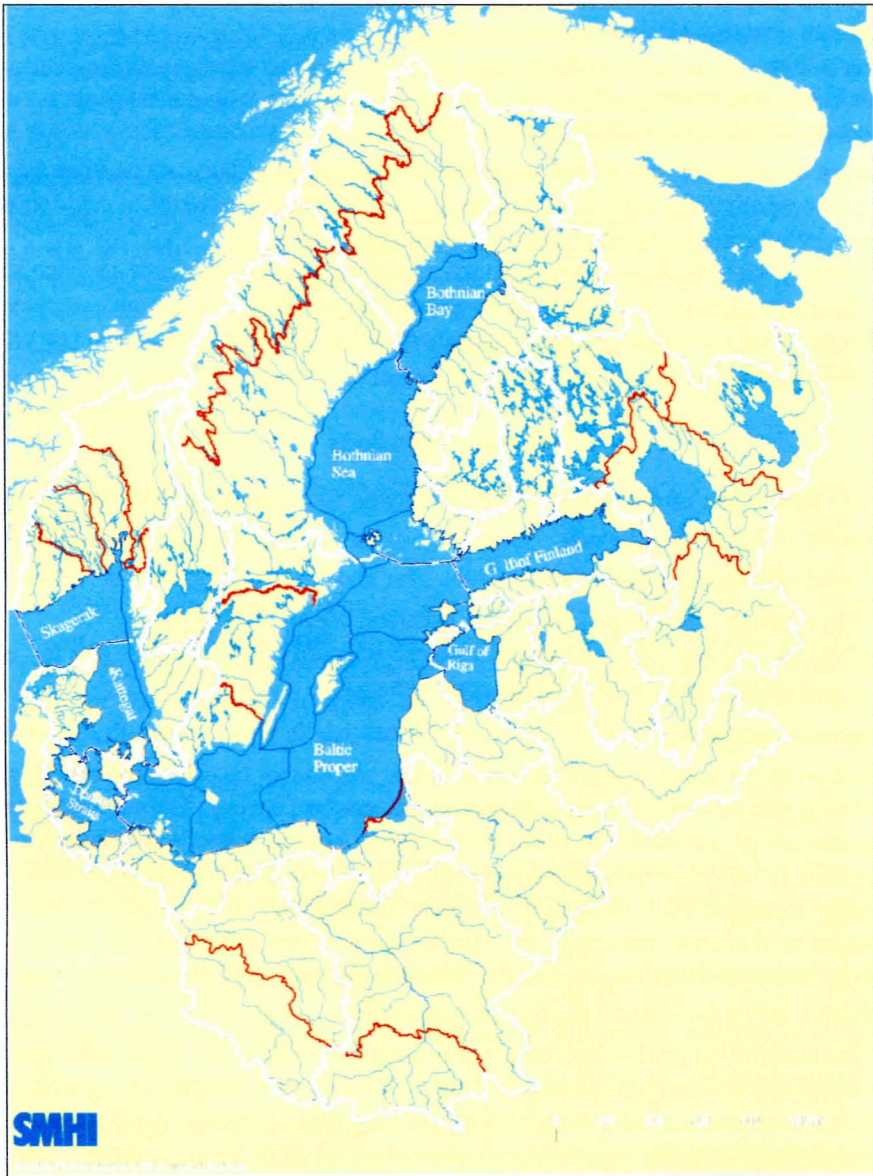
Fig. 4. Catchment area for the Baltic Sea, Skagerrak and Kattegat and the distribution of separate drainage basins (red lines) for which the river runoff forecast model is run. Also shown with thick black lines are the sub-basins for a chemical model. Major rivers are marked with blue lines
