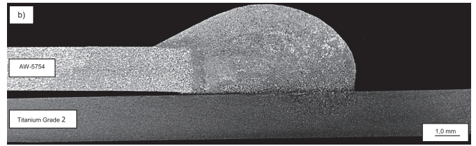
Fig. 3. Macrostructure of the overlap joints of Grade 2 titanium – aluminium alloy AW-5754 braze welded with AlSi5 filler metal \varnothing 2.4 mm, titanium on the top (a) titanium at the bottom (b), chemical etching using Kroll's reagent
