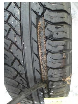
Fig. 7. Circumferential cut with single stream
