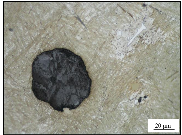
Fig. 5. Structure of a casting soaked at 550°C for 6 h and air-cooled: the largest degree of austenite transformation to fine-acicular ferrite. Etched with Mi1Fe
