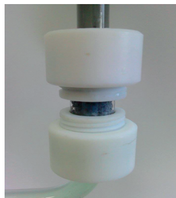
Fig. 2. Reactor for particle coupling in syntactic foam by deposition of nickel
