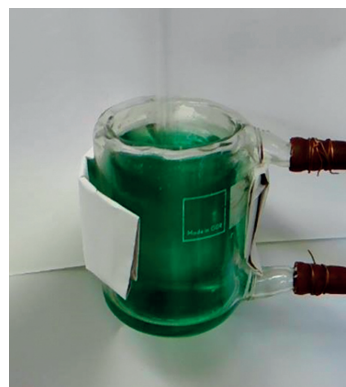
Fig. 1. Water jacket reactor charged with nickel solution. Particles not yet loaded
