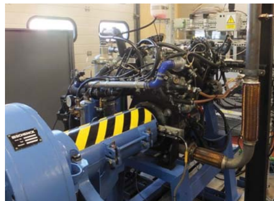
Fig. 1 Inlet manifold (a) and FPT 1.3 MJT engine test rig (b)
