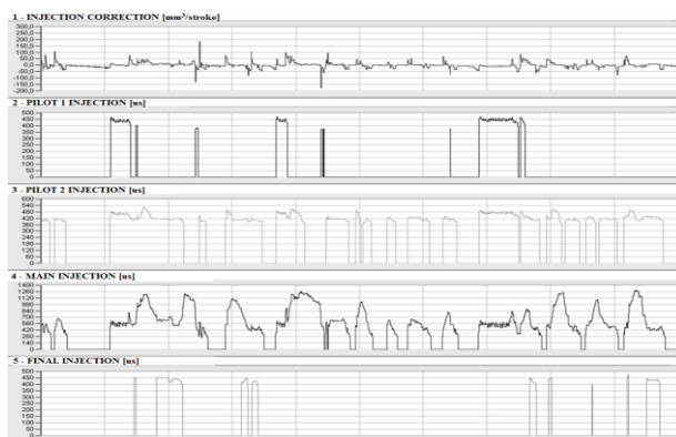
Fig. 7. The recorded signals as a function of time (1 – injection correction, 2 – pilot 1 injection, 3 – pilot 2 injection, 4 – main injection, 5 – final injection)
