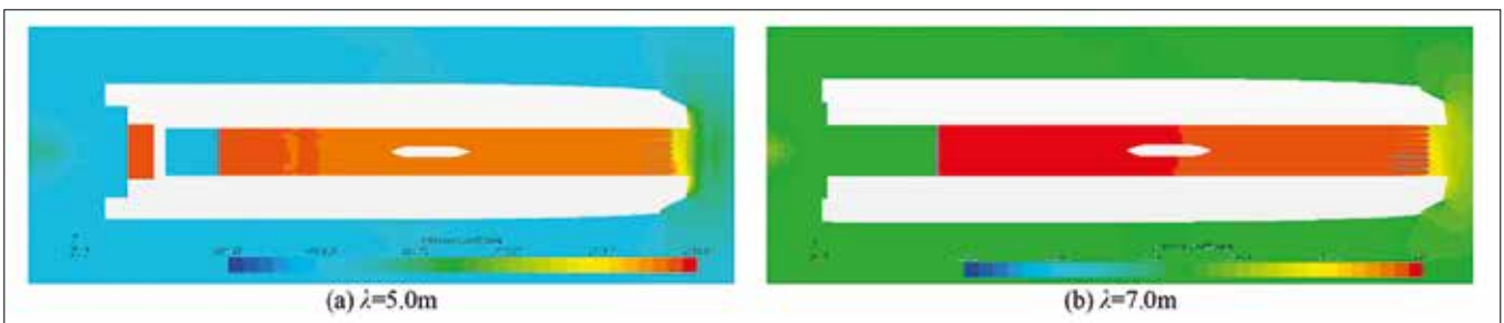
Fig. 23. Pressure distribution of air cushion chamber in the xy plane at speed of V = 2.0\text{m/s}
