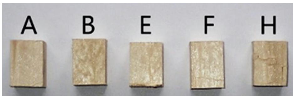
Figure 3: Characteristic failure of test specimens after the immediate compression test along the grain at the crosshead speeds: 0.05 mm/min (A), 0.5 mm/min (B), 5.0 mm/min (E), 9.9 mm/min (F), 50.0 mm/min (H)
