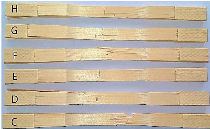
Figure 5: Characteristic specimen fractures after the grain longitudinal tensile strength test at crosshead speed of 2.5 mm/min (C), 3.3 mm/min (D), 5.0 mm/min (E), 9.9 mm/min (F), 15.0 mm/min (G), 50.0 mm/min (H)
