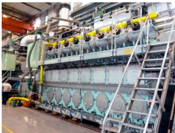
Figure 5. Dual-fuel engine 8L5160DF (MAN Diesel & Turbo, 2013)
