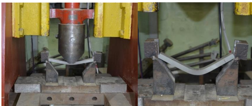
Fig. 5. Bending test of flat sample using drop-weight type impact hammer
