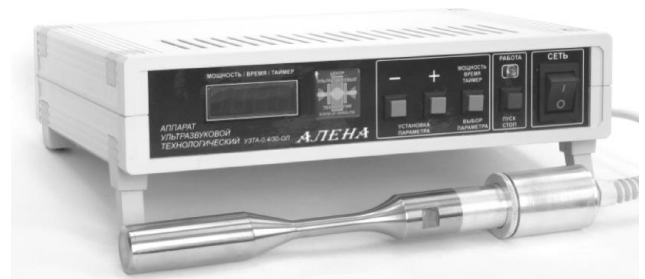
Fig. 8. Appearance of developed concentrating link and ultrasonic apparatus.
