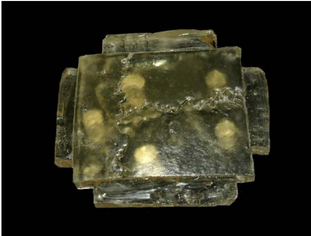
Fig.11. The model of syndesmosis made of epoxy resin Epidian 5
