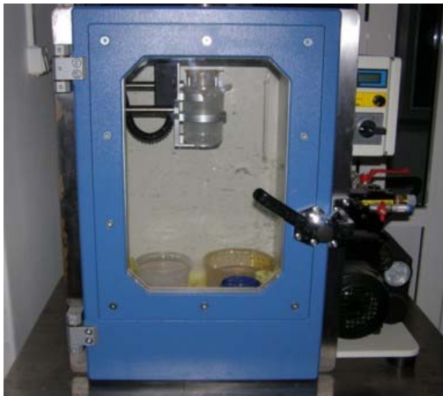
Fig. 8. Vacuum UHG 400 device for vacuum casting
