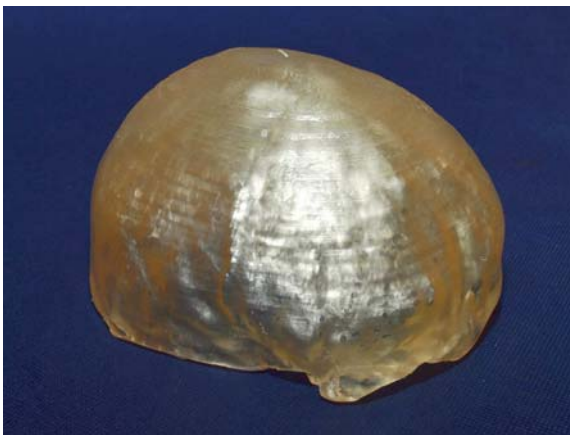
Fig. 2. The 1:1 scale model of a human skull made with SLA method
