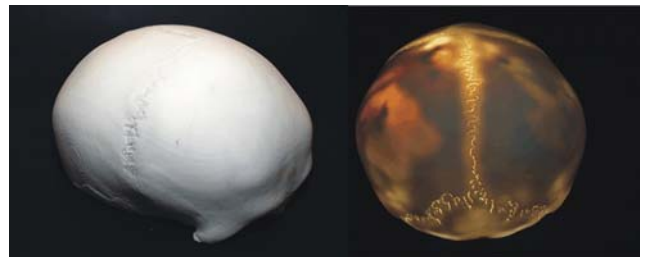
Fig. 4. Models of skull fabricated with SLS method
