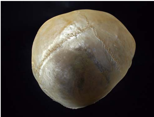
Fig.12. Model made of Epidian 5 resin ready for photoelastic experiment
