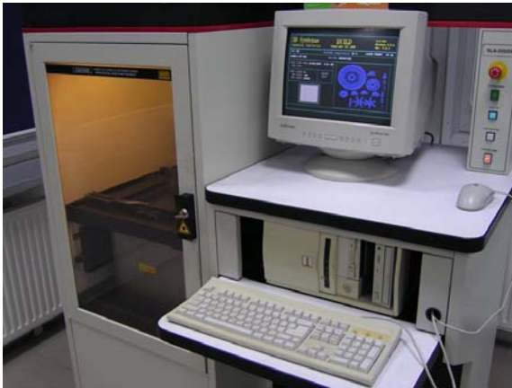
Fig. 1. Stereolithography device - SLA 250/50 (Rzeszow University of Technology)
