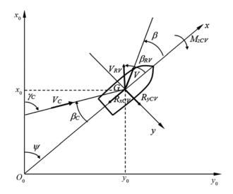
Figure 7. Position and course as well as current direction and speed of the ship's model with drift angle
