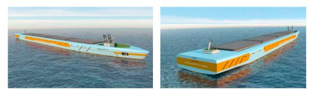
Figure 4. Visualization of the unmanned container, autonomously controlled ( $L_c = 78.75$  m, B = 11.10 m, T = 4.33 m,  $\nabla = 2500$  m<sup>3</sup>)
