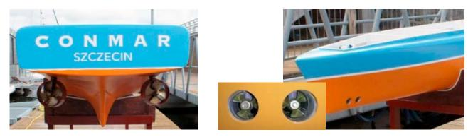
Figure 5. The propulsion system of the autonomous ship model
