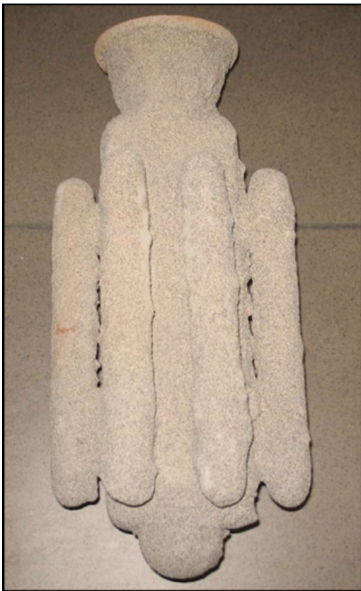
Fig. 1. Ceramic mould for strength test of castings
