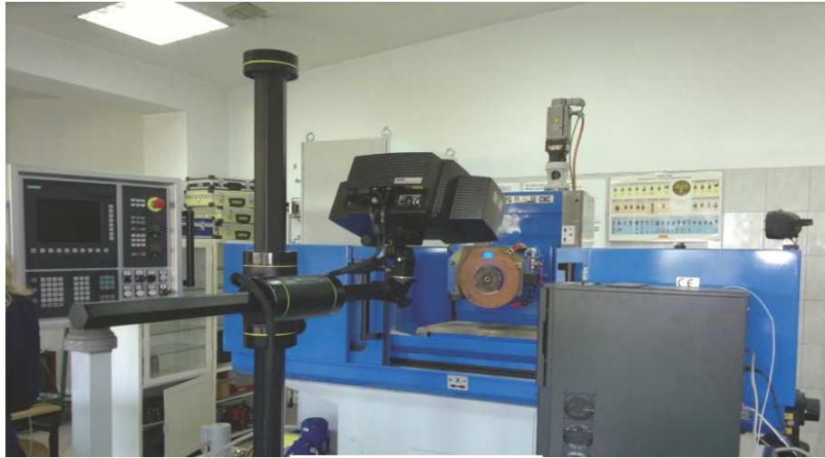
Fig. 1. Triangulation white light scanner ATOS III SO (Small Object) on the laboratory post
