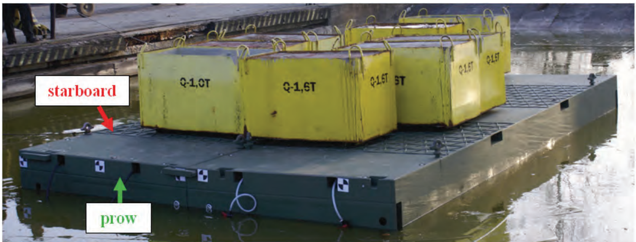
Fig. 2. Experimental examinations of two pontoon bridge cassettes loading
