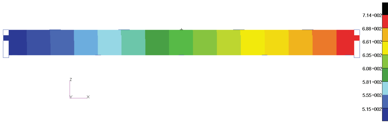
Fig. 6. Pontoons section immersion determined in numerical analysis
