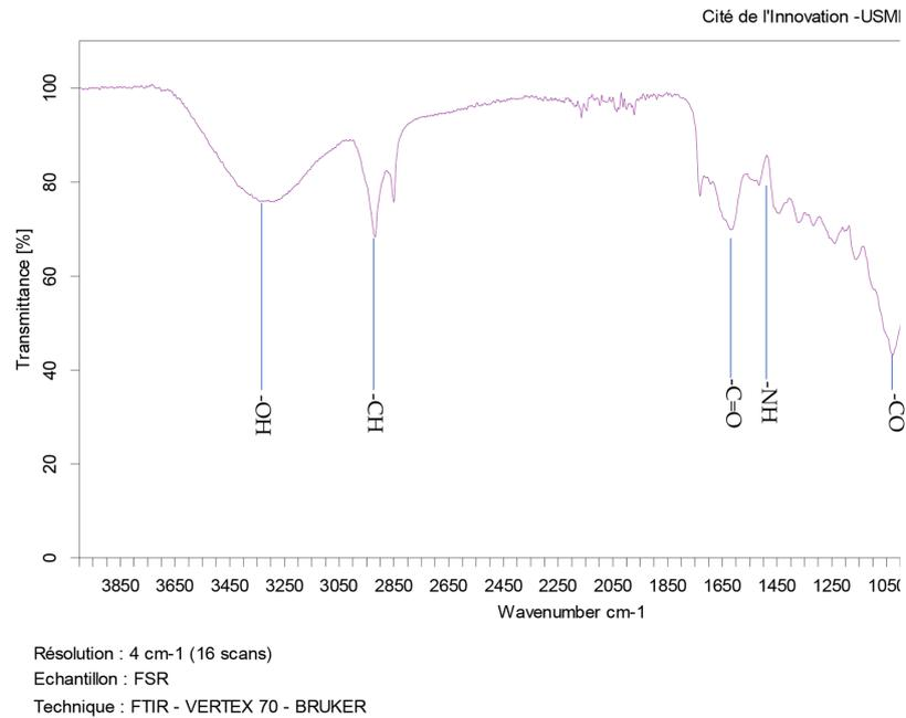
**Figure 4.** Infrared spectrum of the biomaterial AP
