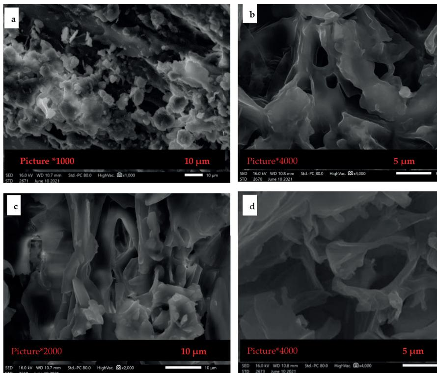
**Figure 6.** Scanning electron microscope observation of the AP biomaterial (a, b before the essential oil extraction; c, d: after the essential oil extraction)
