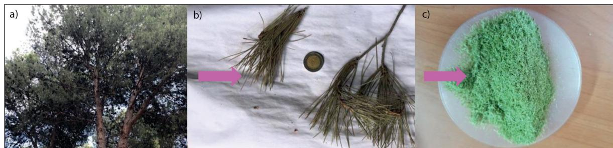
Figure 3. Preparation of the biomaterial (Aleppo pine) (a) Aleppo pine tree, (b) needles, (c) sieved powder
