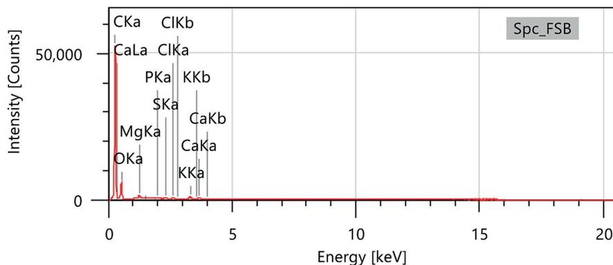
**Figure 7.** Energy dispersive spectrum (EDX) of AP biomaterial
