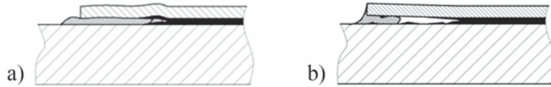
Figure 2. Previous repair methods: a) bonding after deflection and cleaning, b) bonding without deflection.
