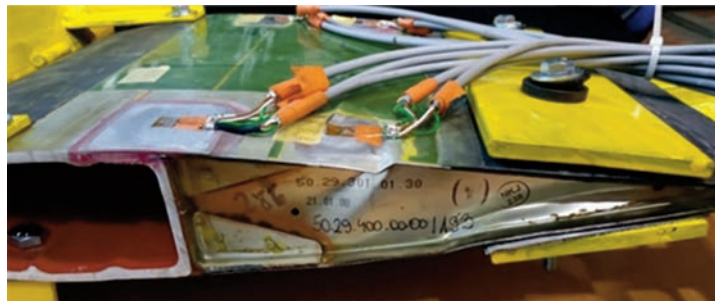
Figure 16. Section side view after static destruction.
