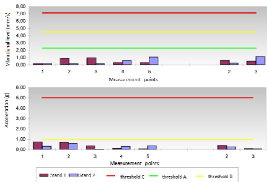
Fig. 6. Velocity and the accelerations measures on gear box vs ISO value
