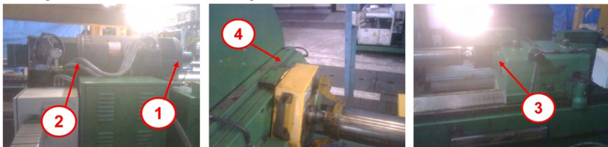
Fig. 3. Accelerometers position on grinding machine
