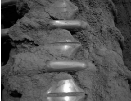
Fig. 5. A view of the chain wheels during the wear tests in the presence of quartz abrasive
