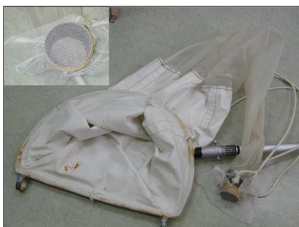
Photo 1. Sample collecting drag – constructed by the staff of the Department of Marine Ecology and Environmental Protection of the West Pomeranian University of Technology Szczecin
