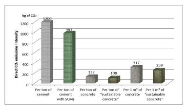
Fig. 1. Typical direct CO2 intensity - cement and concrete
