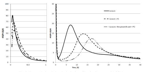
Fig. 7. Heat evolution during the hydration of Portland cement with SCMs
