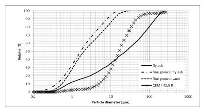
Fig. 2. Particle size distribution of cement and SCMs
