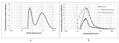
Fig. 5. Coefficient of incremental surface activity  $K_{isa}$  of cement (a) and SCMs (b)
