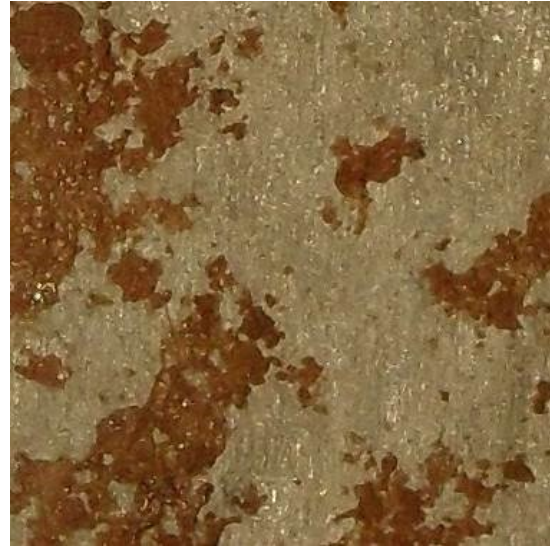
Figure 13. Specimen AW-6060 with alkyd varnish +30% volcanic tuff – 630 hours.
