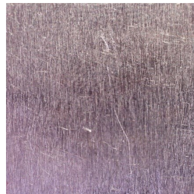
Figure 6. Surface of a raw aluminium specimen.
