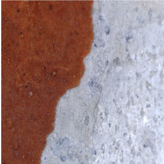
Figure 12. Specimen AW-6060 with alkyd varnish +40% brick dust – 630 hours.
