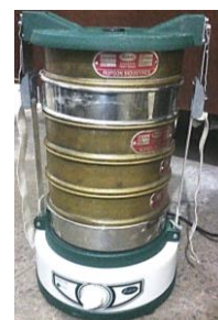
Fig. 13. (a) Sieve vibrator (b) Sieves with retained plantain flour
