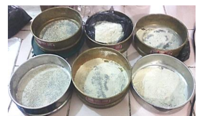
Fig. 13. (a) Sieve vibrator (b) Sieves with retained plantain flour
