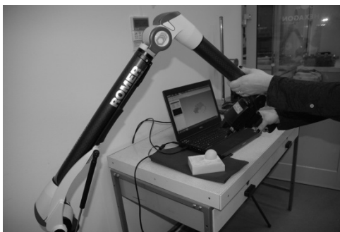
Fig. 5. Measurement with the Romer Arm 7320SI with HP-L-20.8 laser scanner in 3D Reshaper software
