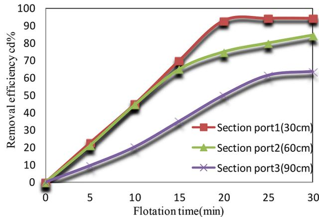
Figure 10. Changes in removal rates over time and at various sampling port during flotation by MBs at fixed (Flow rate 0.50 L/min,  $C_{Cd(II)}$  30 mg/L,  $C_{SDS}$  15 mg/L, and PH 7.2)
