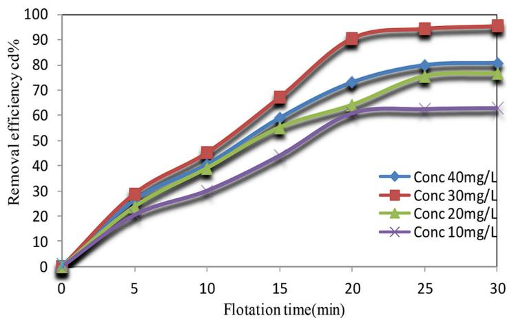
**Figure 4.** Changes in removal rates over time and at various initial Cd (II) values during flotation by MBs at fixed ( Flow 0.50 L/min,  $C_{SDS}$  15 mg/L, PH 7.2 and  $S_p$  30 cm)
