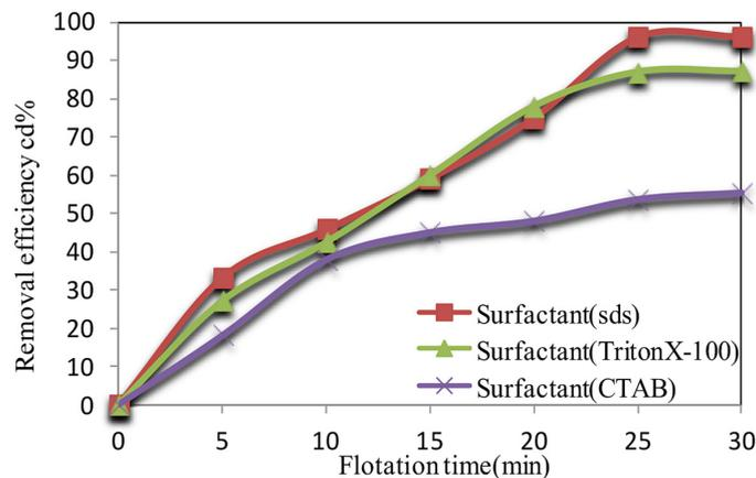
Figure 11. Change of removal rates with time at different type of surfactant at same  $C_{sur}$  15 mg/L with fixed (Flow 0.50 L/min,  $C_{Cd(II)}$  30 mg/L, PH 7.2 and Sp 30 cm)
