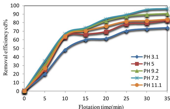
**Figure 2.** Changes in removal rates over time and at various initial PH levels during flotation by MBs at fixed conditions (Flow 0.50 L/min,  $C_{SDS}$  15 mg/L,  $C_{Cd(II)}$  30 mg/L, and  $S_p$  30 cm)
