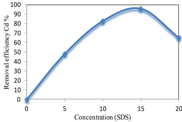
**Figure 7.** The relationship between Cd(II) removal efficiency and various initial concentrations  $C_{SDS}$  at fixed (Flow rate 0.50 L/min,  $C_{Cd(II)}$  30 mg/L, PH 7.2, and  $S_p$  30 cm)
