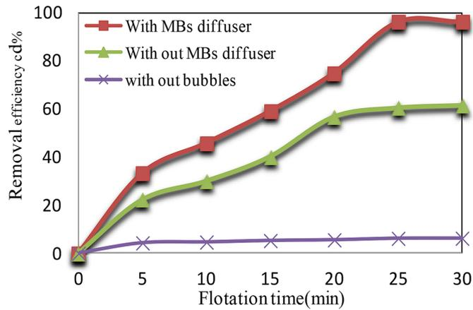
**Figure 12.** Change of removal rates with time at different MBs and without its, with fixed (flow rate 0.50 L/min,  $C_{Cd(II)}$  30 mg/L,  $C_{SDS}$  15 mg/L, and PH 7.2)
