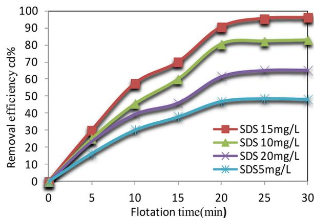
**Figure 6.** Changes in removal rates over time and at various  $C_{\text{SDS}}$  during flotation by MBs at fixed (Flow rate 0.50 L/min,  $C_{\text{Cd(II)}}$  30 mg/L, PH 7.2, and  $S_p$  30 cm)
