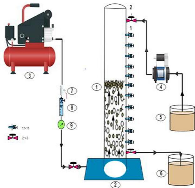
**Figure 1** shows a schematic of a system for micro-bubble air flotation in a laboratory; (1) micro-bubble diffuser, (2) flotation column (3) an air compressor; (4) a feed pump; (5) a feed tank; (6) an effluent tank; (7) a valve; (8) an air rotameter; (9) a pressure gauge; and 1 (1–11) sampling taps, 2 (1–3) columns, and diffuser valves
