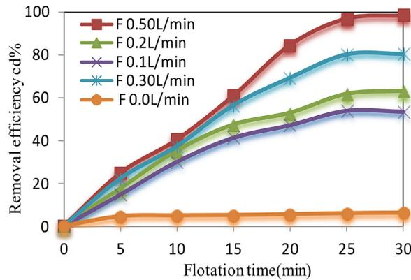
**Figure 8.** Changes in removal rates over time and at various flow rate during flotation by MBs at fixed ( $C_{Cd(II)}$  30 mg/L,  $C_{SDS}$  15mg/L, PH 7.2, and  $S_p$  30 cm)
