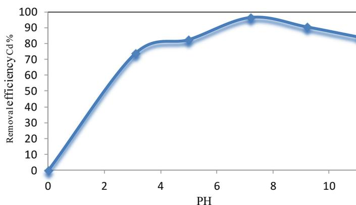
**Figure 3.** The relationship between Cd(II) removal efficiency and various initial PH solution at fixed (Flow 0.50 L/min,  $C_{SDS}$  15mg/L,  $C_{Cd(II)}$  30 mg/L, and  $S_p$  30 cm)
