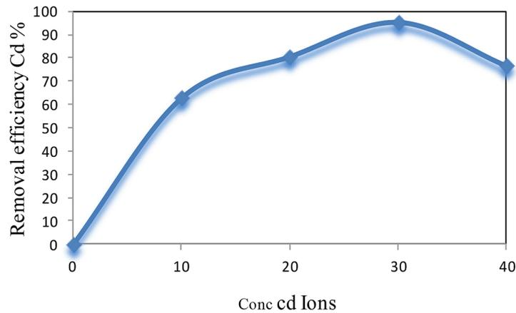
**Figure 5.** The relationship between Cd (II) removal efficiency and various initial concentrations Cd(II) values at fixed (Flow rate 0.50 L/min,  $C_{\text{SDS}}$  15 mg/L, PH 7.2, and  $S_p$  30 cm)
