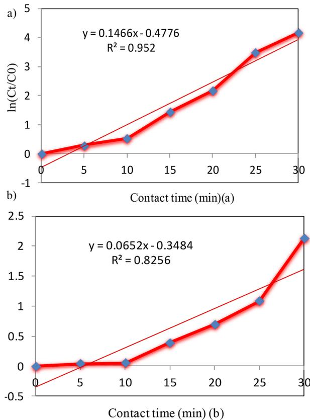
**Figure 13.** Time dependency of the estimated and experimental values of  $C_{Cd(II)}$ , (a) first order, and (b) second order
