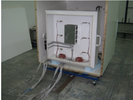
Fig. 2. Photo of the heating box inside the body model
