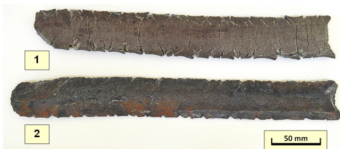
Fig. 3. Effect alloy FeAl during rolling without shields (1) and using shields (2)
