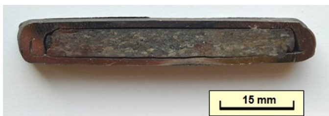
Fig. 2. FeAl method to shield the alloy during rolling
