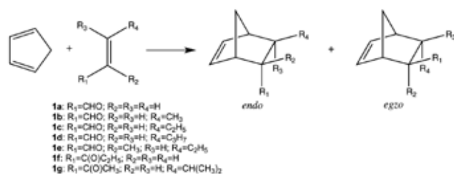
Fig. 4. Diels-Alder reaction between cyclopentadiene and various dienophiles
