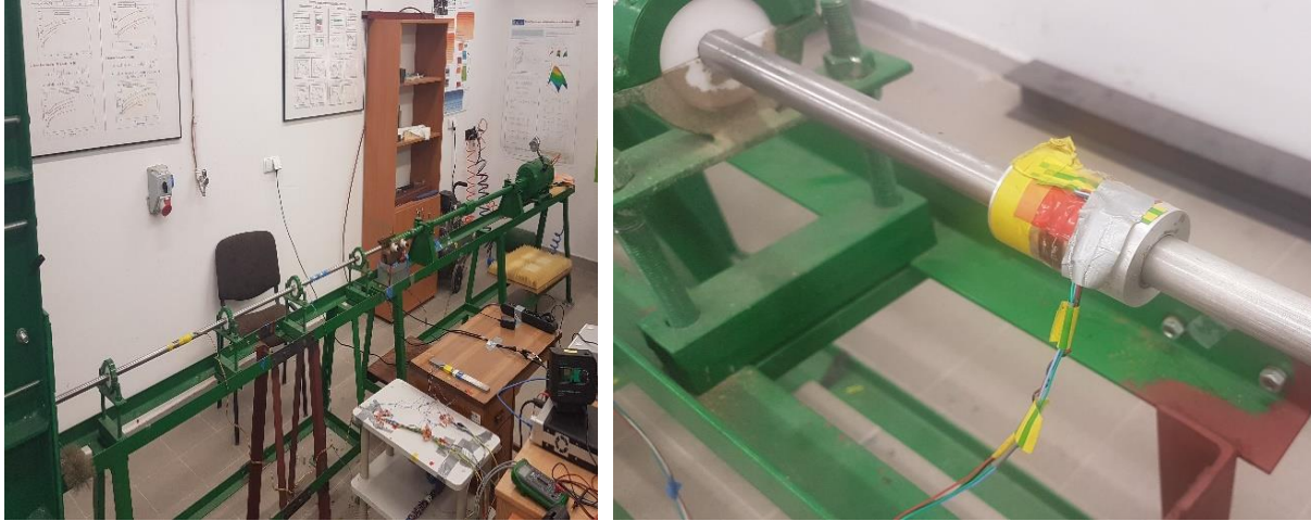
Fig. 4. General view of a SHPB in MUT. Fig. 5. Specimen in rigid casing (with strain gauge).
