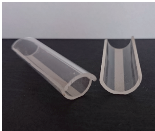
Fig. 1. Quartz holder for heating the material in a CVD oven designed for the purpose of the experiment
