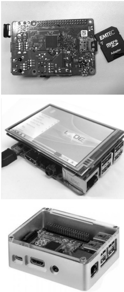
Fig. 13 My microcomputer open Hardware RaspBerry PI 2b with WIFI micro USB. O.S. Raspbian (Linux Rasperry-Debian)
