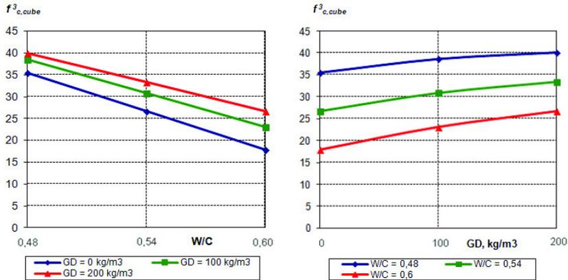
Fig. 2. Graphic dependencies of concrete compressive strength at the age of 3 days with the use of granite dust
