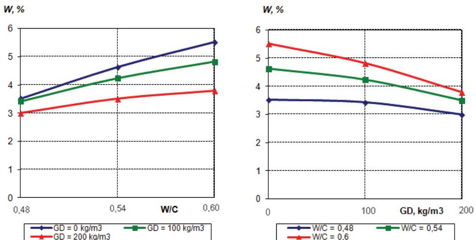
Fig. 5. Concrete water absorption diagram using granite dust
