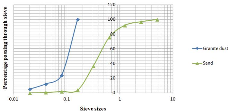
Fig. 1. Particle size distribution of granite dust and sand
