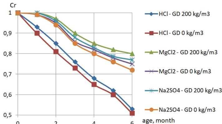
Fig. 7. Coefficients of corrosion resistance of concrete filled with granite dust
