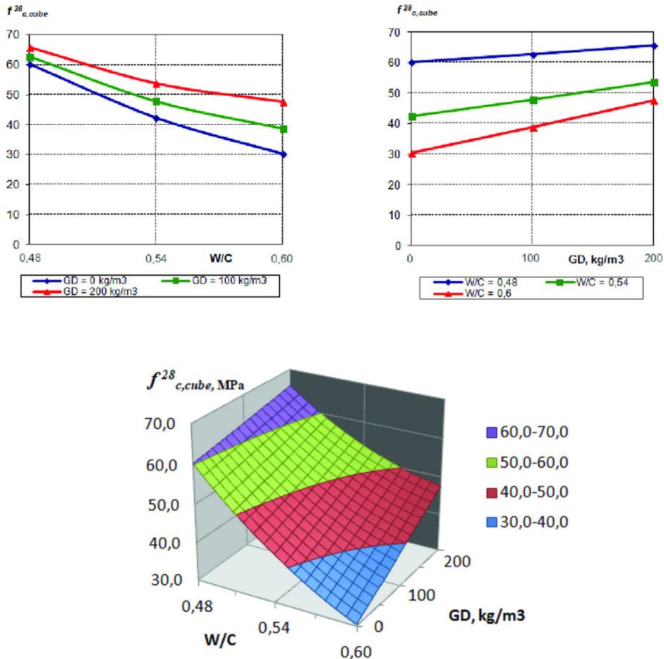
Fig. 3. Graphic dependencies of concrete compressive strength at the age of 28 days with the use of granite dust
