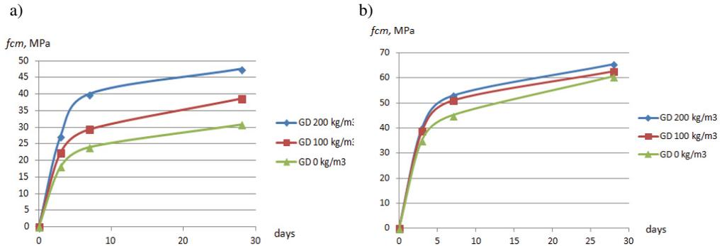
Fig. 4. Kinetics of strength change of concrete filled with granite dust: a)  $W/C = 0.60$ ; b)  $W/C = 0.48$
