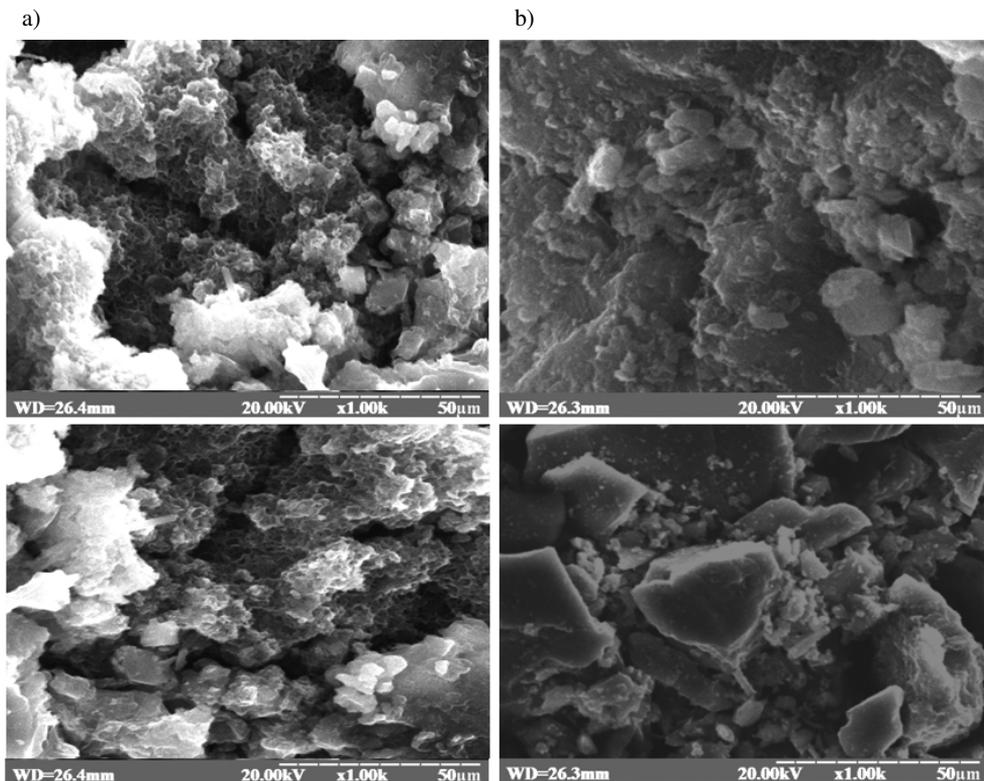
Fig. 6. Microstructure of cement stone without GD (a) and with the use of GD (b), at the age of 28 days
