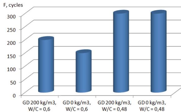
Fig. 8. Frost resistance of concrete
