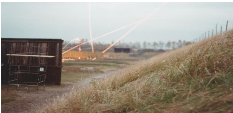
Picture 8. A burst of 4 shots to a distance of 100 m. T-45 bullets ( 7.62 \times 39 mm intermediate cartridge) fired from an AK carbine
