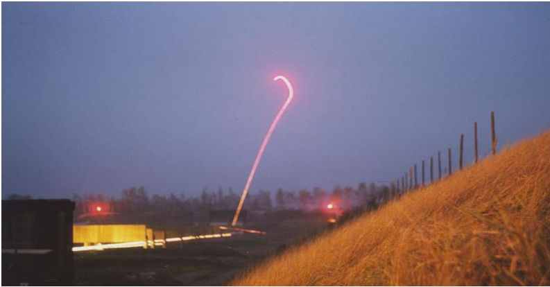
Picture 6. A burst of 3 shots to a distance of 100 m. T-45 bullets ( 7.62 \times 39 mm intermediate cartridge) fired from an AK carbine
