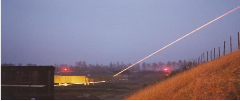
Picture 4. Flight trajectory of a single T-45 bullet ( 7.62 \times 39 mm intermediate cartridge) and its ricochet Shooting at targets 100 m away
