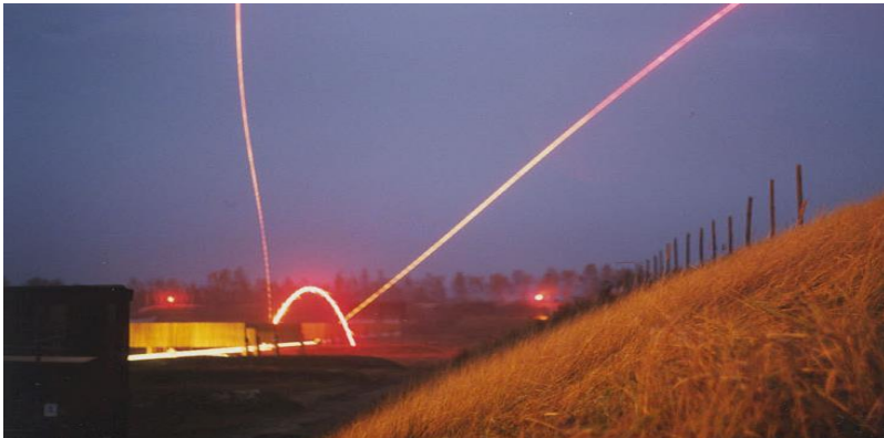
Picture 7. A burst of 4 shots to a distance of 100 m. T-45 bullets ( 7.62 \times 39 mm intermediate cartridge) fired from an AK carbine
