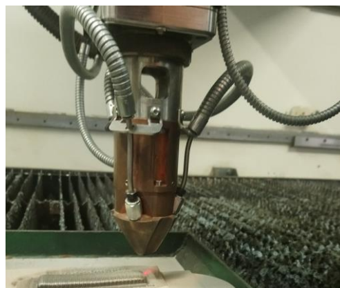
Fig. 1. Deposition process of Inconel 625 metallic powder
