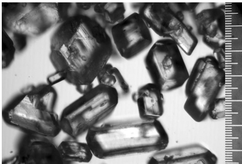
Figure 2. The image of screened commercial nitramine after 1 h of spheroidization using the ultrasonic method (spacing between minimum graduation marks is 10 \mu\text{m} ; working fluid was water)
