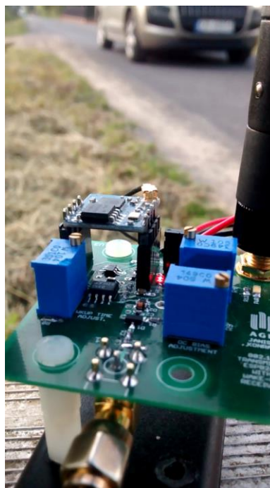
Fig. 14. Frame from a video of the test with vehicle moving with 74 km/h speed. Red LED is indicating that transmitter is woken-up
