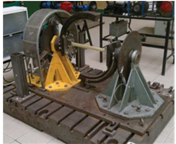
Fig. 7. The view of the device type ZP-1 with the mounted composite sample
