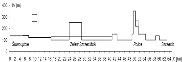
Figure 5. Width of the waterway (W) in function of its length (X) for two analyzed Alternatives I and II
