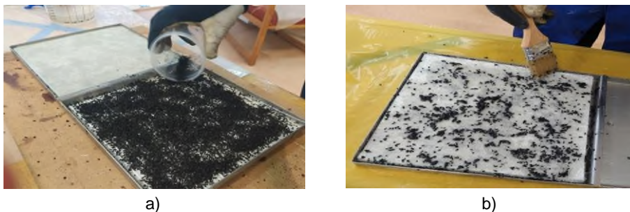
Fig. 1. Composite material with the addition of recycle a) as a sandwich layer b) as an addition to the composite matrix
