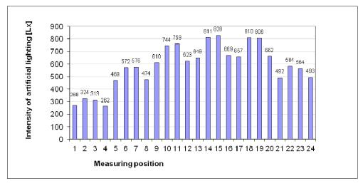
Fig. 5. General lighting intensity at worktops fixed to seats located on the subsequent height levels in the room during a presentation and with maximum artificial light (*own research*)
