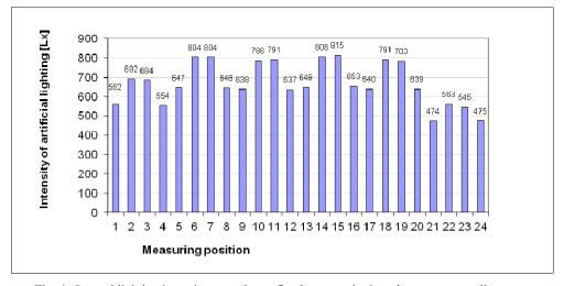
Fig. 4. General lighting intensity at worktops fixed on seats in the subsequent ascending rows with full artificial lighting (*own research*)
