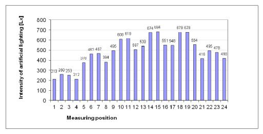
Fig. 6. General lighting intensity on worktops fixed to seats located at subsequent height levels in the room during presentation and with half of the maximum artificial light (*own research*)
