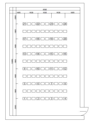
Fig. 1. Scheme of the didactic room with marked measuring stations where general lighting was measured (*own research*)
