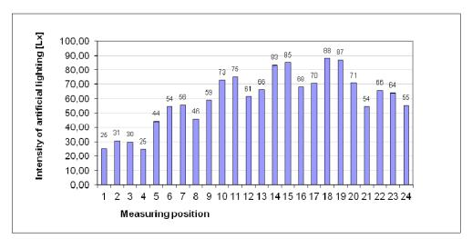
Fig. 7. General lighting intensity on worktops fixed to seats located at the subsequent height levels in the room during presentation and with minimum artificial light (*own research*)
