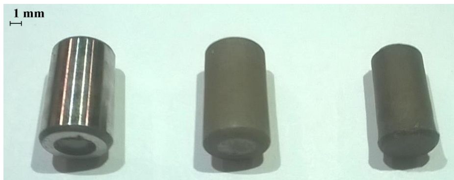
Figure 2. Rollers of dismantled CBK 171 tapered bearing treated with acids
