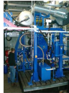
Fig. 7. Test engine for calibration of calculation model
