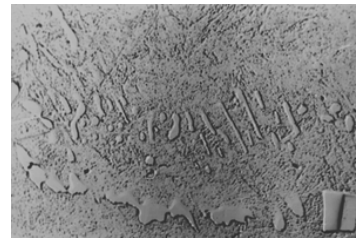
Fig. 10. Micrograph of cast iron, t_A = 1020^\circ\text{C} , t_w = 820^\circ\text{C} , \tau_w=16\text{ min} , TEM, microscopic magnification 3400x
