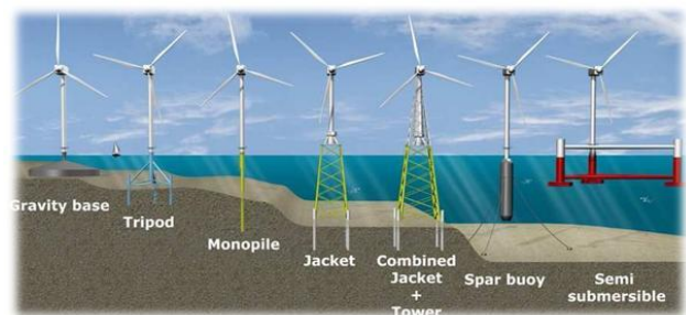
Figure 2. Offshore floating wind turbines – methods of anchoring on the seabed and floating structures [2]
