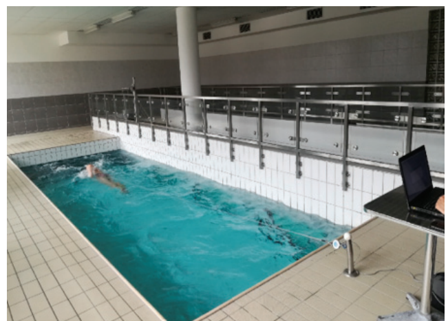
Fig. 1. Measurement of force during a 40-second all-out tethered front crawl arm stroking test
