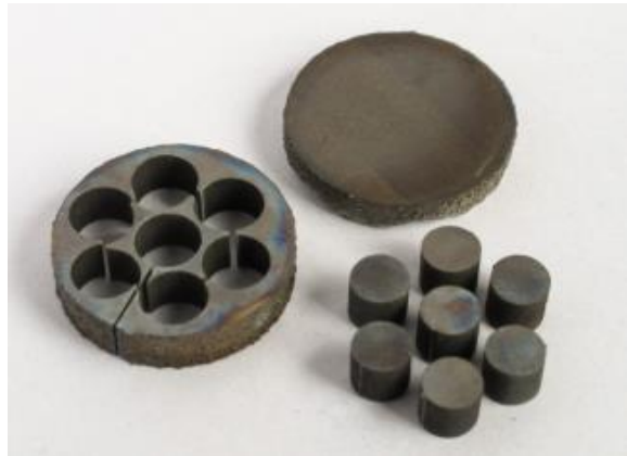
Fig. 4. Test specimens made using the electrical discharge machining
