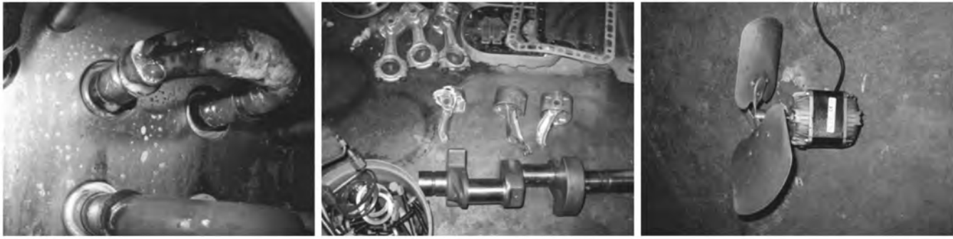
Fig. 1 Examples of refrigeration systems elements failures
