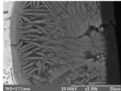
Fig. 5. Micrograph by SEM obtained in secondary electrons of surface layer of steel GradeB A284 specimen, ESA on the air: anode — Al; I = 2...2,5 \text{ A} ; \tau = 300 \text{ sec} and sequent LT on the air ( W_p = 2,6 \text{ GW/m}^2 ).
